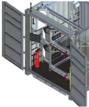
Container interior: two-level rack and discharge units
