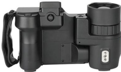
Rear view: touch screen, controls and connectors
