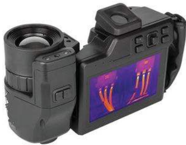
Thermal overlay on the touch screen, with the viewfinder above
