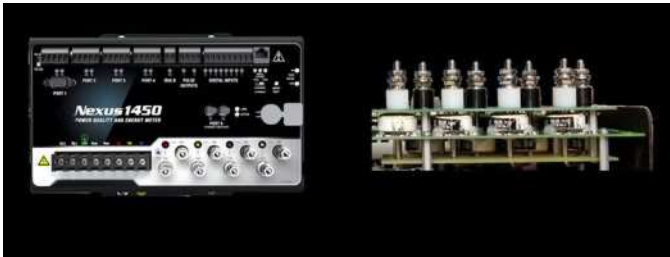
Meter base with the two current sensing stages and the six communication ports
