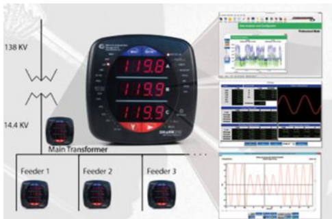
Voltage and frequency recording at the main transformer and the feeders
