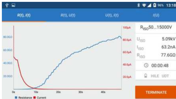
Real-time resistance and current graphs in the mobile application during the test
