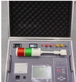
Control unit with printer, display and output and measurement terminals
