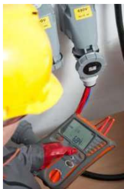
Loop measurement at a 690 V industrial socket with the AMZC-305
