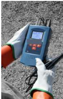
PDRM-10A micro-ohmmeter taking a field measurement
