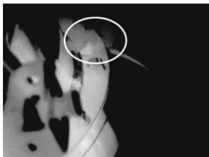
Leak plume as seen by the cooled detector
