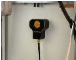
SonoTEV Pro sensor magnetically attached to a panel
