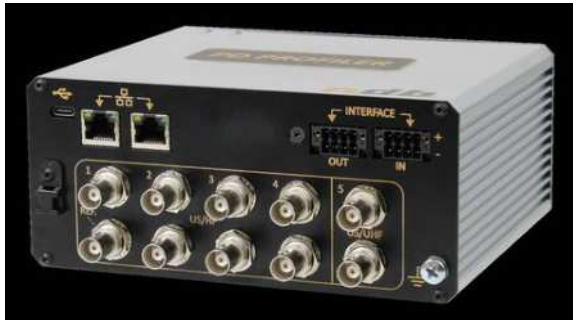
Acquisition unit with BNC inputs and daisy-chain ports
