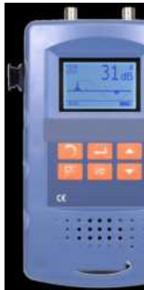
PXDP-II detector with its partial discharge analysis display
