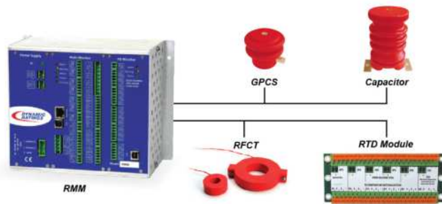
Detection zone: coupling capacitors + RTD-PD module
