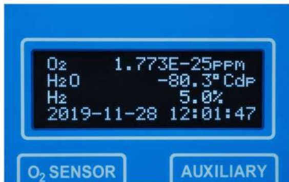
OLED display: O 2 , dewpoint and H 2 content on one screen
