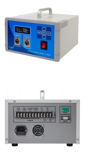
For customers requiring seamless integration into their product or process, the Rapidox 2100 can be supplied as an OEM solution. Please contact Amperis for further information. Zirconia oxygen sensors are particularly suitable for monitoring inert atmospheres in aggressive industrial applications within manufacturing processes; this includes high temperature locations and vacuum atmospheres.
