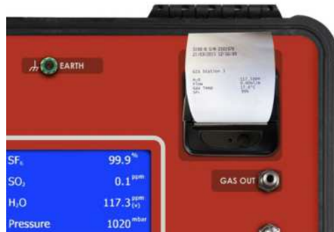
Integrated thermal printer: test reports on demand
