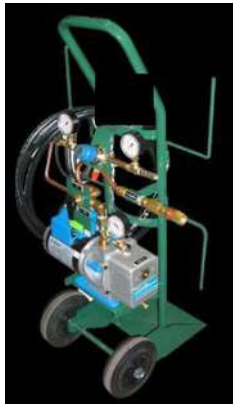
Valve and gauge assembly of the ARFU-2
