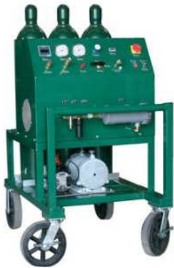
On-board rack for three SF 6 cylinders and control panel
