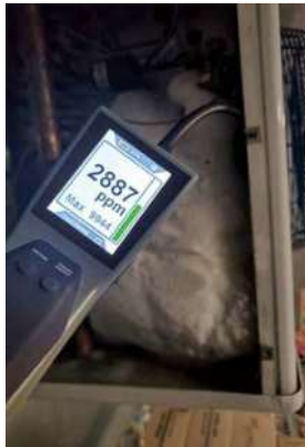
The detector, with its flexible probe and the concentration display
