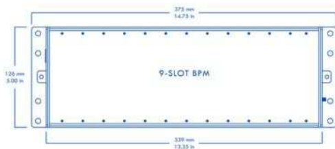
9-slot BPM chassis: 375 × 126 mm front panel (14.75 × 5.00 in) and 339 mm on the lower dimension line (13.35 in), with the same 143 mm depth (5.62 in).
