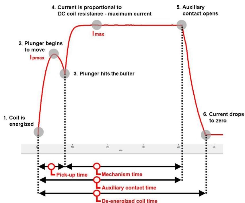
Figure 3. Coil current specific points and measurement parameters
