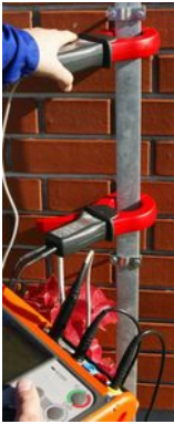
Double-clamp method: earth resistance without disconnecting the installation
