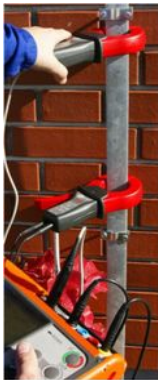
Double-clamp measurement on an earth rod, without disconnecting the installation
