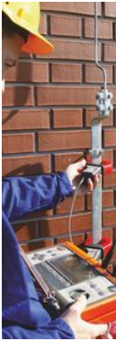
Double-clamp method: earth resistance without disconnecting the installation
