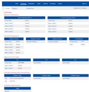
Web dashboard: measured and calculated temperatures, load currents and insulating-paper ageing in real time.
