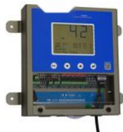
Surface panel mounting in an existing cabinet (IP31/NEMA-2).
