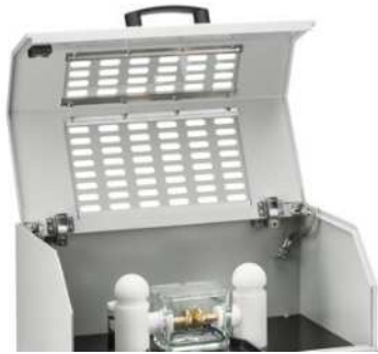
Test chamber with the glass vessel and the electrodes
