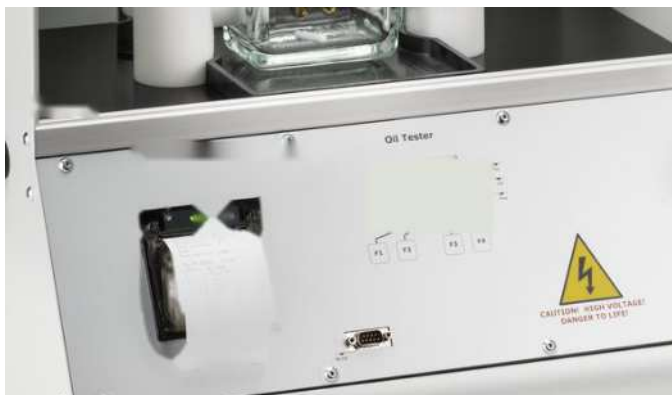
Built-in thermal printer and graphic display of the panel
