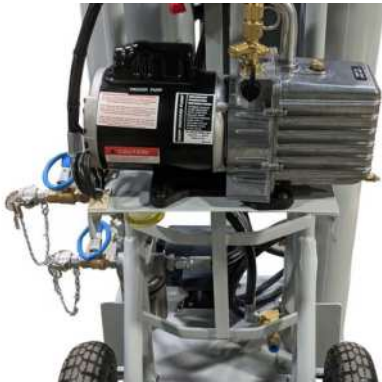
High-vacuum pump and filtering assembly
