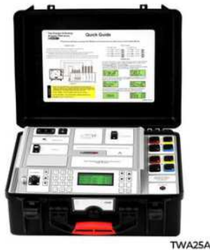
Front view of the TWA Standard Series, with keypad, LCD display and transport case.
