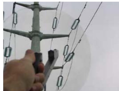
Application example: to detect corona effects on overhead electrical insulators.
