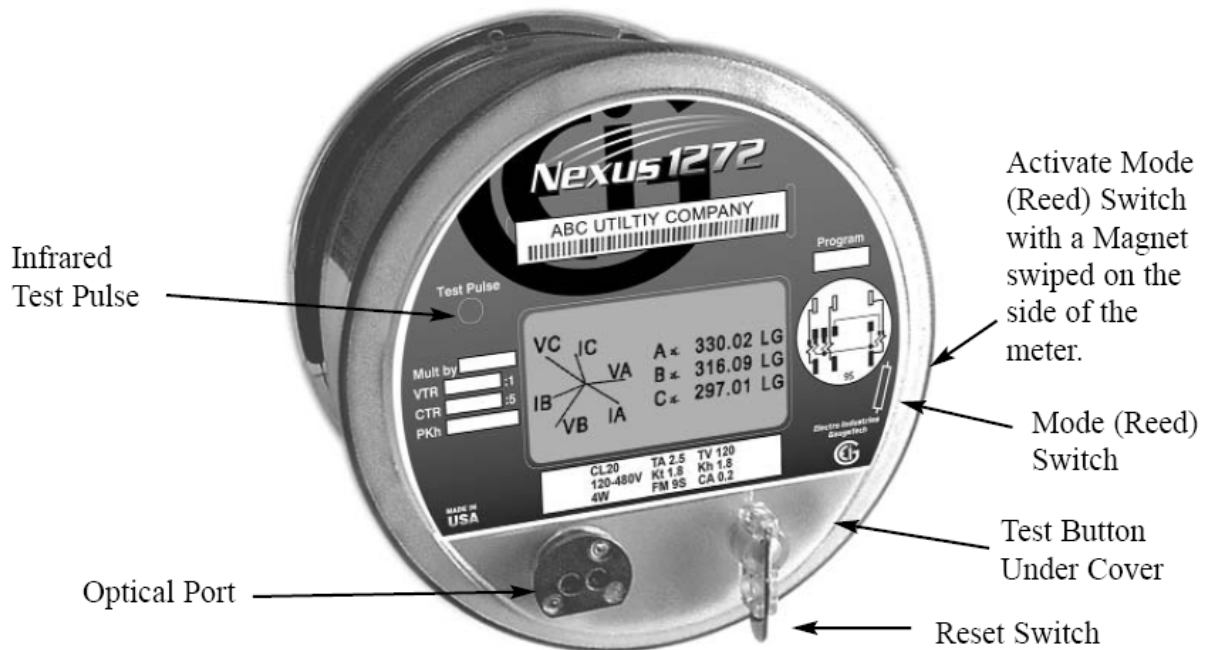
Figure 3.2: Nexus 1262/1272 Switches and Indicators
