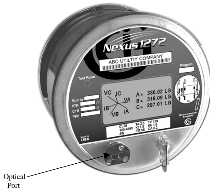
Fig. 5.2: Nexus 1272 Optical Port
